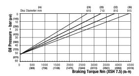
Maximum Braking Force XSH 7.5: 11.2kN (2517.86 lbf) Minimum Pressure for full retraction: 63 bar (914 psi) Weight of caliper and thruster - 13.62kg (30.03 lb)
