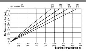
Maximum Pressure 7 bar (102 psi) Maximum Braking Force = 1.9kN @ 7 bar (427.14 @ 102 psi) Weight of caliper and thruster - 9.52kg (20.99 lb) Weight of thruster only - 0.3kg (0.66 lb) Volume displacement of thruster at full stroke = 64ml (2.16 fl oz)
