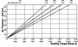
Maximum Pressure 7 bar (102 psi) Maximum Braking Force = 3.6kN @ 7 bar (809.31 @ 102 psi) Weight of caliper and thruster - 10.37kg (22.86 lb) Weight of thruster only - 1.15kg (2.54 lb) Volume displacement of thruster at full stroke = 150ml (5.07 fl oz)
