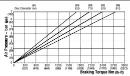
Maximum Pressure 7 bar (102 psi) Maximum Braking Force = 6.9kN @ 7 bar (1551.18 @102 psi) Weight of caliper and thruster - 10.54kg (23.24 lb)
