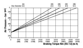
Maximum Braking Force XS 7.5: 11.2kN (2517.86 lbf) Minimum Pressure for full retraction: 5 bar (73 psi) Weight of caliper and thruster - 14.12kg (31.13 lb)
