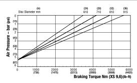
Maximum Braking Force XS 9.6: 14.3kN (3214.77 lbf) Minimum Pressure for full retraction: 6.5 bar (94 psi) Weight of caliper and thruster - 14.32kg (31.57 lb)
