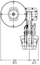
Weight actuator only - 8.7kg (19.18 lb) Weight of controller - 5.5kg (12.13 lb)
