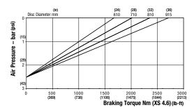
Maximum Braking Force XS 4.6: 6.8kN (1528.70 lbf) Minimum Pressure for full retraction: 3 bar (44 psi) Weight of caliper and thruster - 13.72kg (30.25 lb)
