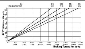
Maximum Pressure 7 bar (102 psi) Maximum Braking Force = 11kN @ 7 bar (2472.89 @ 102 psi) Weight of caliper and thruster - 11.28kg (24.87 lb)
