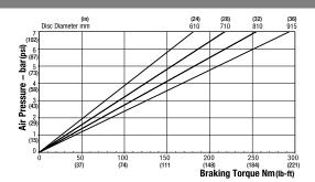
Maximum Pressure 7 har (102 psi) Maximum Braking Force = 0.74kN @ 7 bar Weight of caliper and thruster - 9.56kg (21.07 lb)
